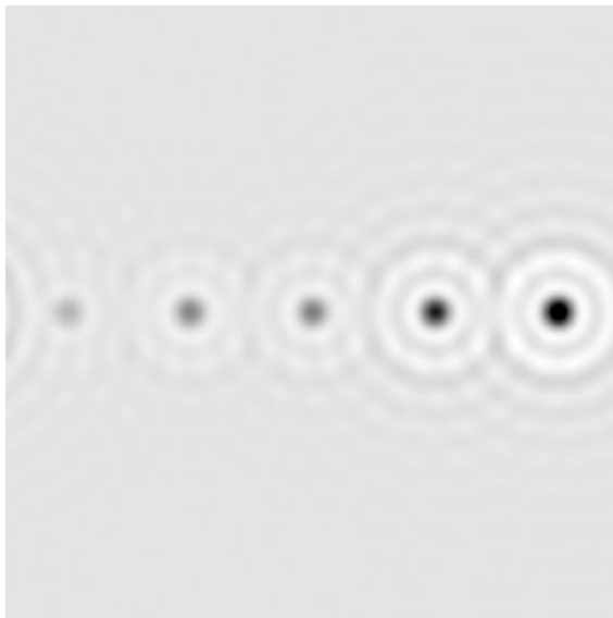
Fig. 5.12 The coherent bright field phase contrast image of five isolated single atoms and an incident electron beam energy of 200 keV. The electron optical parameters are spherical aberration C_s = 1.3 mm, defocus \Delta f = 700 Å and an objective aperture of 10.37 mrad (Scherzer conditions). This was calculated with a sampled image of 512 \times 512 pixels. Atomic number Z = 6 (C), 14(Si), 29(Cu), 79(Au), 92(U) (left to right). The image ranges from 0.72 (black) to 1.03 (white)
